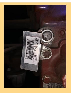
In the picture above, note that you can see the original maker's tag below right of the servicer's tag. This shows the valve model and part number. The serial number should be there also, just not visible in the picture. All of that data plus dates is required to "associate" this valve to a car.
