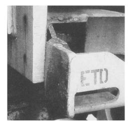
EOT bracket with additional side offset for end sill clearance.
