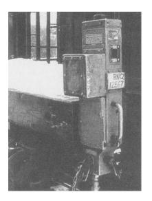
Bracket mounted to bottom of buffer with EOT in place.
