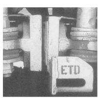
EOT bracket offset to the side, and lowered for additional clearance.
