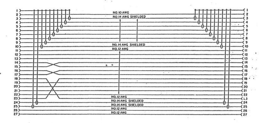
FIGURE 2.3IC - WIRING DIAGRAM - 27 POINT COMMUNICATION JUMPER CABLE, CAR - CAR
