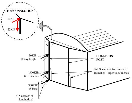
Figure 3 - Schematic of Collision Post Loads for Coach Cars
