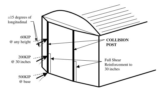
Figure 2 - Schematic of Collision Post Loads for MU and Cab Cars (Cab End Only)
