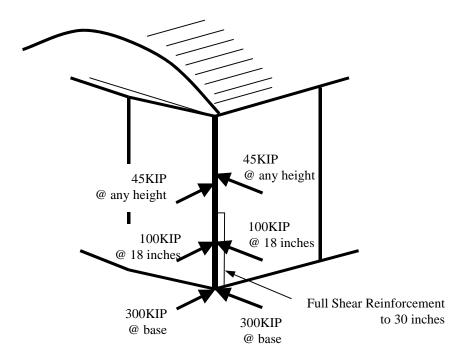
Figure 5 - Schematic of Corner Post Loads for Cab Ends of MU Cars and Cab Cars
