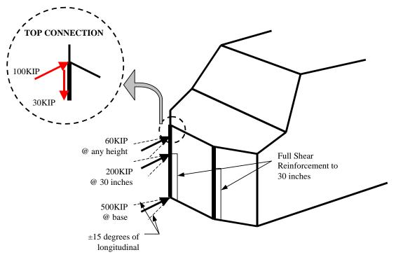
Figure 1 - Schematic of Collision Post Loads for Non-Passenger-Carrying Locomotive
